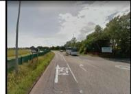
Bus stop layby on southeast side of road to be removed and replaced with a 3 metres wide shared use footway / cycle route. New bus stop border to be installed in the carriageway.
